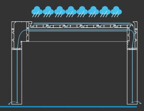
In our new generation SKYFREE models, we made special additions to the water drainage solutions in the rail-panel junction points and side cover designs. The water, which is directed sideways from the panel-rail junction point over the panel, is transferred to the double grooves in the rail for water discharge. If under heavy rain conditions, excessive water puddle occurs and the water overflows to the sides, it cuts the water on the side covers and directs it to the gutters.
