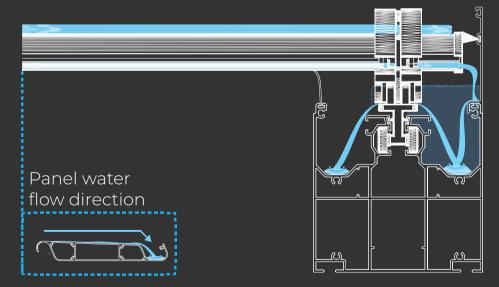
In our new generation SKYFREE models, we designed two-sided slots that move through the rails, in order to keep the movement of the cars perfectly always, to add weather strip to the rails. With these slots, dust and small particles are prevented from entering the car path. The movement of the panel continues with the quality of the first day.
