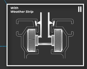
The new **SKYFREE** rail side covers are specially designed both aesthetically and technically. Cover profiles have been added to cover the detailed system view from the sides. Weather strips added to the inside of these profiles prevent dust and small particles from entering the system.
